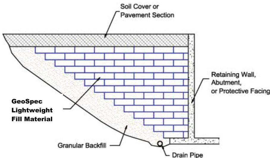
Since GeoSpec fill material density is low relative to standard aggregate backfill materials, vertical stresses that develop behind a retaining wall or abutment are much lower than for an aggregate backfill. Lateral forces exerted by GeoSpec fill material are also minimal because the Poisson's ratio of GeoSpec fill material within its
